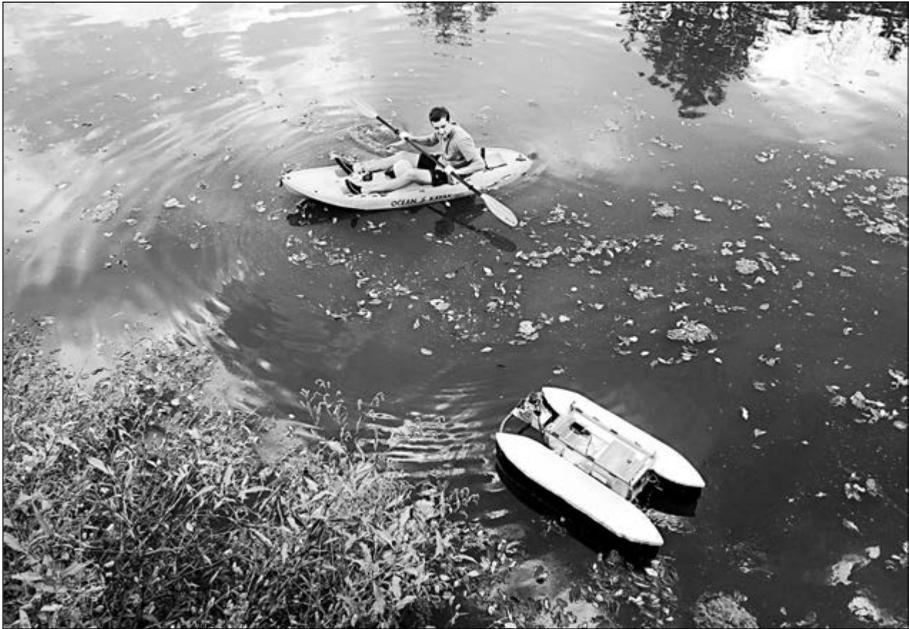
J. “Wes” Anderson, a member of the Villanova team, keeps an eye on the boat as it is put through a series of tests. The craft, which carries a camera, laser, and other electronics, is a prototype of a 16-foot version. ED HILLE / Staff Photographer
